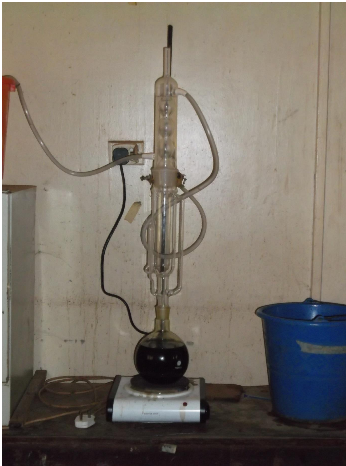
Plate 1: Preparation of plant extracts using Soxhlet apparatus
