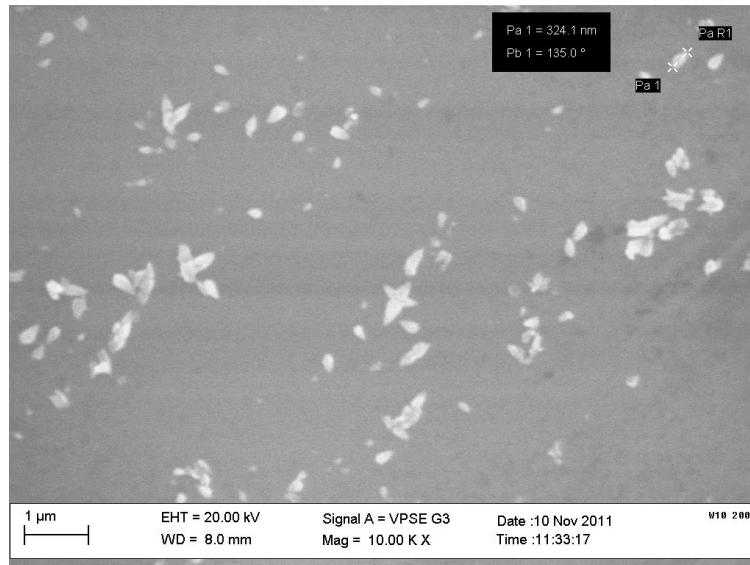
Fig.9. SEM of W10200 grown at pH 10.0 and annealed at 200°C
