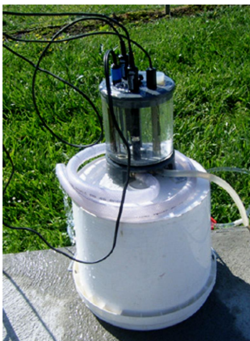
Fig.3.2 Flow cell used to monitor the field parameters.
