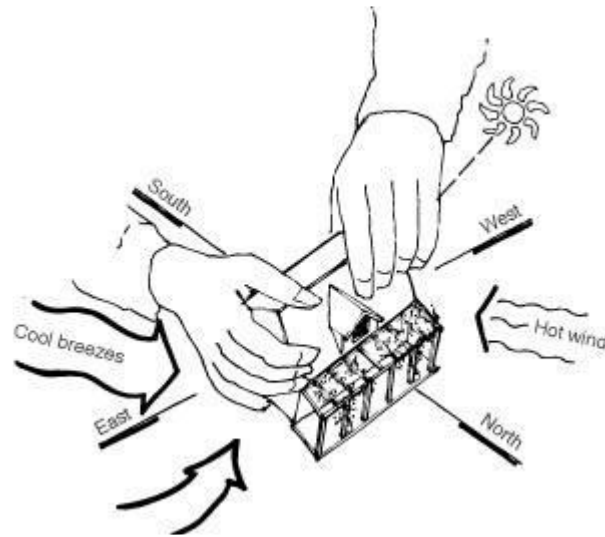
Fig 4.8: illustrates orientations and its effects on ventilation
