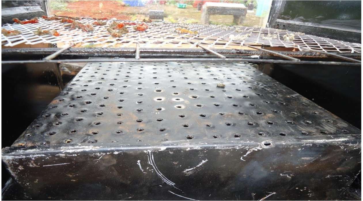
Fig 30: Interior of the passive solar dryer with the heat storage incorporated
