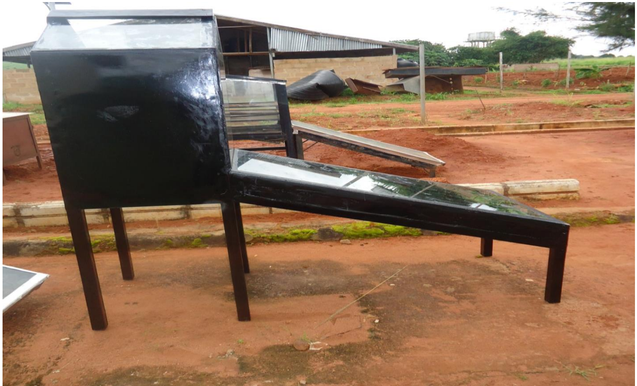
Fig 28: Side view of the constructed solar dryer
