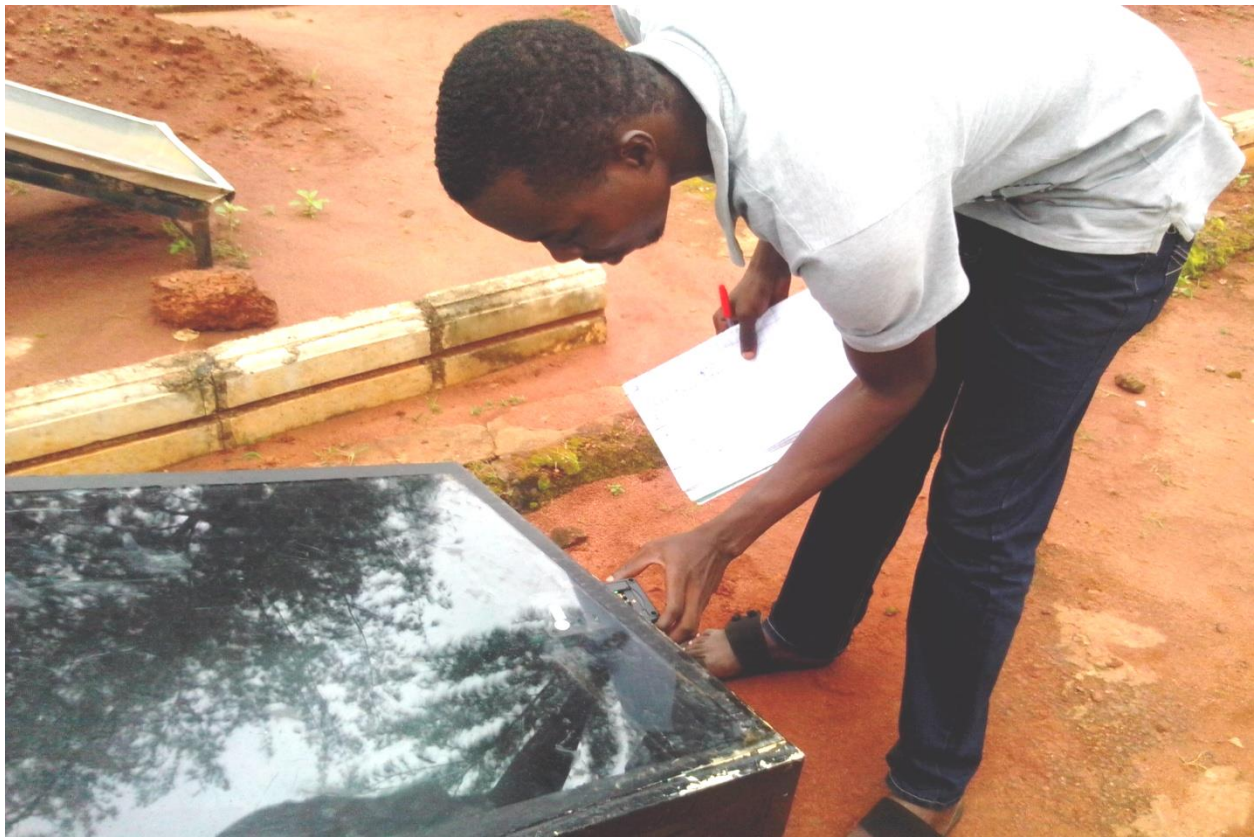
Fig28: Temperature measurement of the collector
