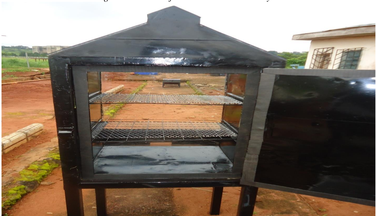
Fig 29: Interior of the passive solar dryer without the heat storage incorporated
