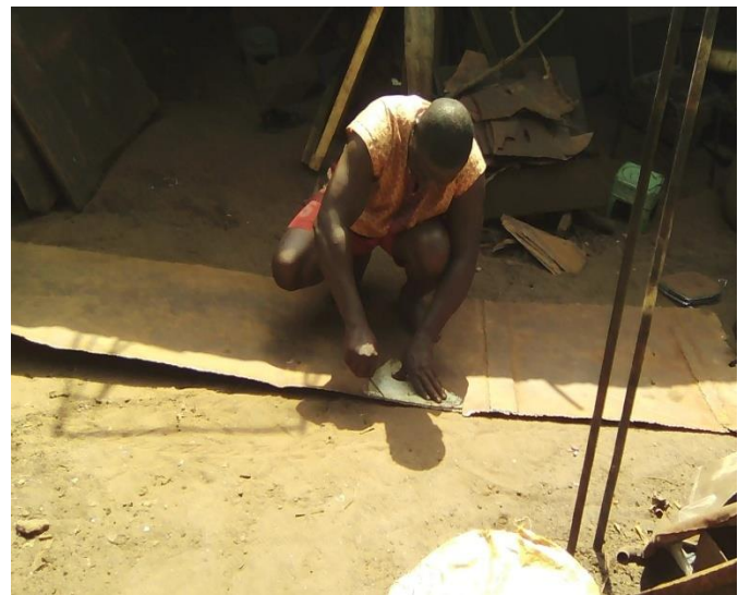
Plate Twelve: Showing Mr. Onyeibor Isaac drawing a pattern on a metal sheet.
